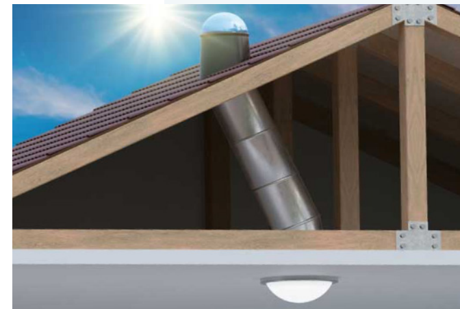
Solar tunnel and how it directs light into living space through attic SOURCE: EnergySage
